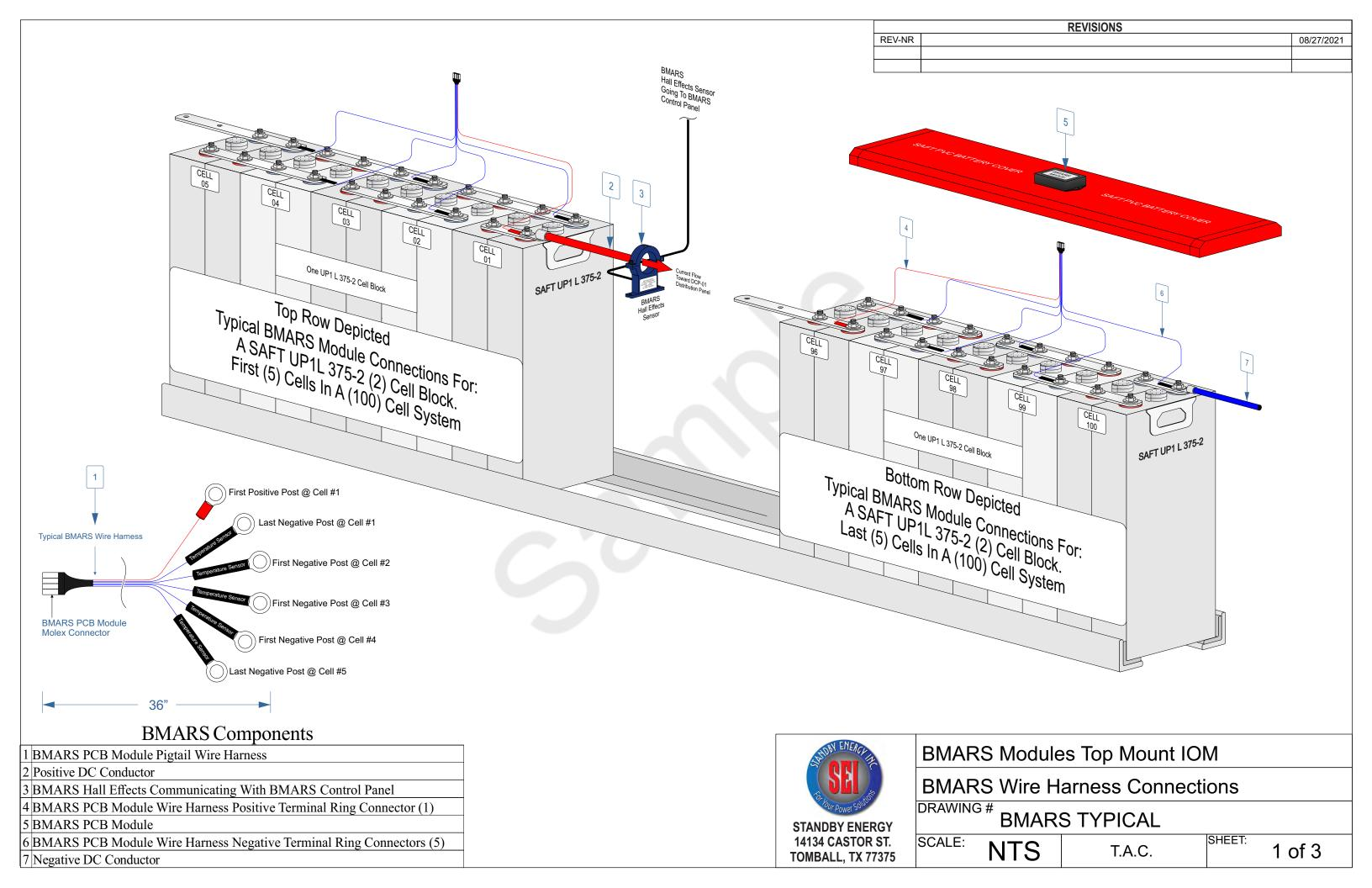
Please note that Temperature Sensors need to run along the bus bars as shown in the picture below. This is so that the red battery covers will fit onto the top of the batteries for safety.
