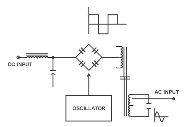
Since all regulating and current limiting functions are inherent, the need for control feedback loops is eliminated. The absences of these feedback loops provides a very reliable and stable voltage that is fixed and not subject to change due to component failure. The ferroresonant inverter is insensitive to non-linear or high crest factor loads making this type of system ideally suited for computer backup.
