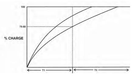
$T_1$ : directly relates to the current capacity of the charger. (Double the current capacity of the charger and  $T_1$  is reduced by a factor of approximately 2.)
